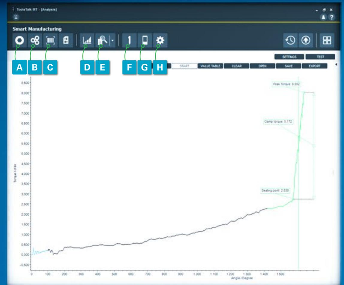
**F TOOL SETTINGS:** Keep track of the quality of your tools, by analyzing the tool lifetime performance and setting calibration intervals.
