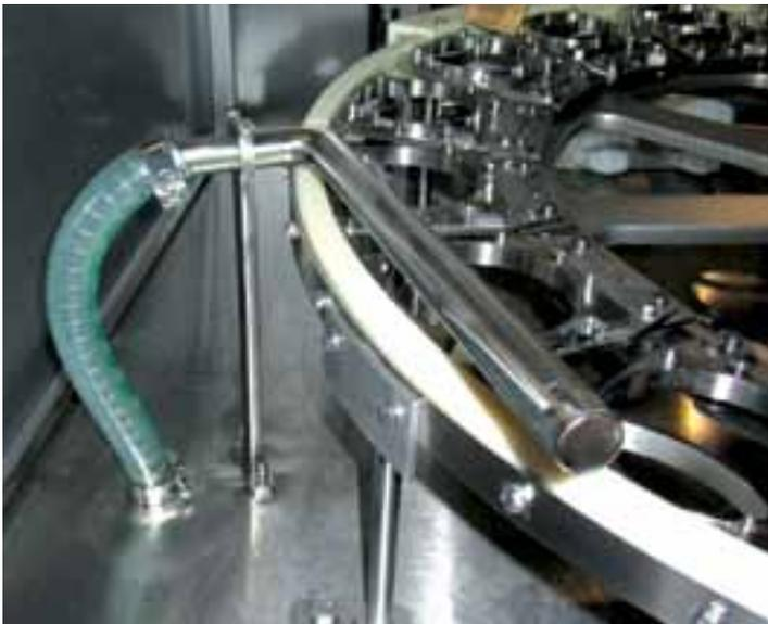
Air Solution de-germination device in filler carousel.
