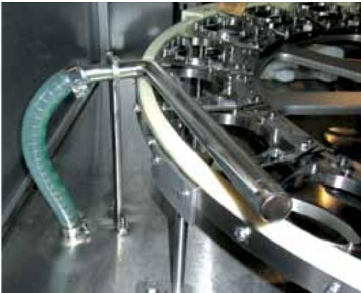
Air Solution de-germination device in filler carousel.
