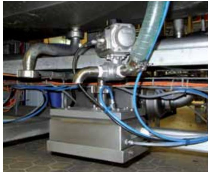
The fogging unit is installed under the packaging machine.
