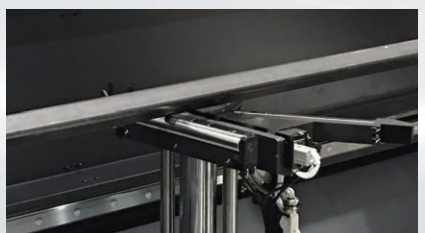
3 Flat support Flat roller follows the shape of material, so that the material will not sag from its own weight.
