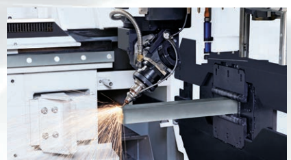
8 Bevel cutting Improved quality of processed components thanks to unsurpassed 3D laser cutting.
