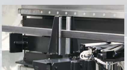
5 Horizontal support OPTION Horizontal support for long beams and small pipes by roller to prevent material displacement.
