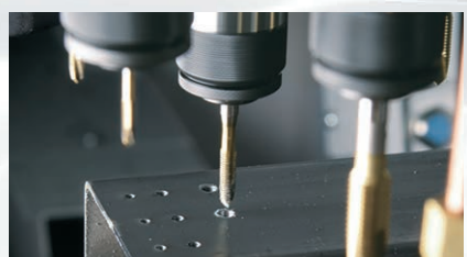
7 Tapping unit OPTION Perform 3D laser cutting, tapped hole preparation and tapping- all in the same machine. The hole to be tapped is cut by the laser and then tapped for shorter production lead time and higher productivity. [Max. M12 (1/2 UNC and UNF)]
