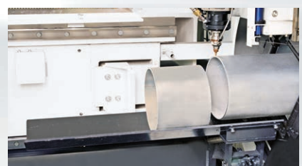
9 Parts catcher Can catch a finished part up to 1000 mm (39.37") long and remove from machine.
