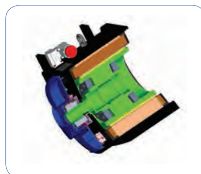
Design of a Cartridge DDR motor (CDDR)
