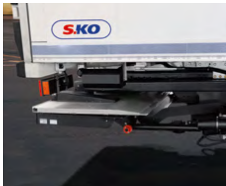
Retractable tail lift for comfortable and safe loading away from the ramp.
