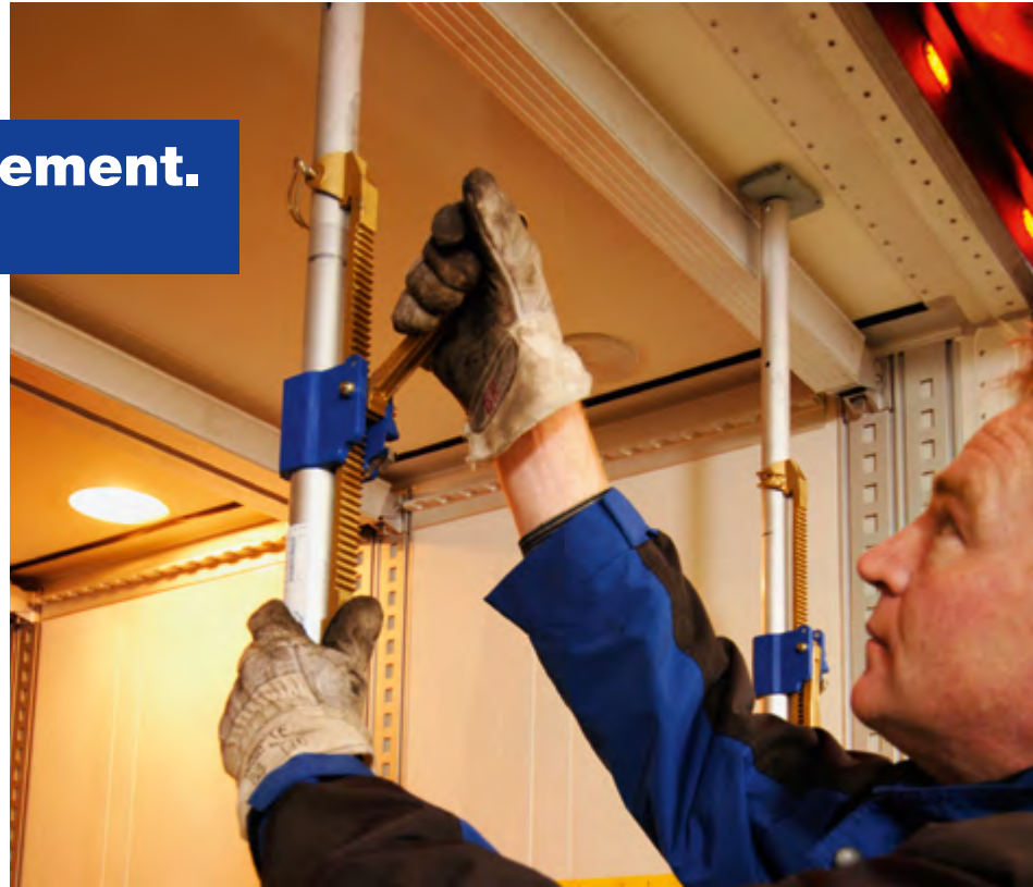
Flush-mounted load securing rails for horizontal clamping bars and tensioning belts.
