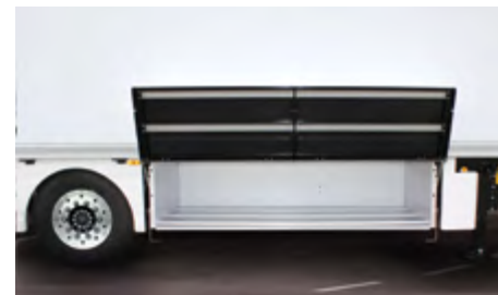
Pallet box for 36 pallets all flaps – even the wheel arches – can be individually lifted up and held in place.
