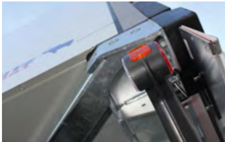
Protection when docking: Diagonal corner reinforcements divert impact forces on the body into the chassis. This protects the body and avoids deformations at the rear.
