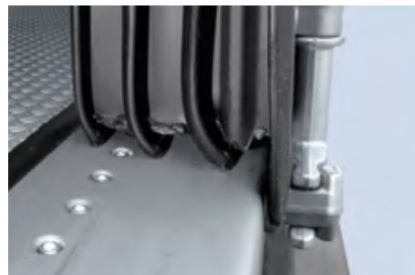
Four-lip door seal to perfectly seal the box body.
