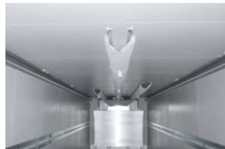
Uniformly cool: flexible cooling ducts for the distribution of cold air at roof level.
