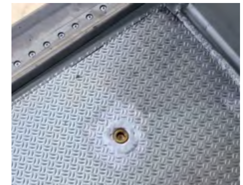
The drain in the floor pan simplifies cleaning.
