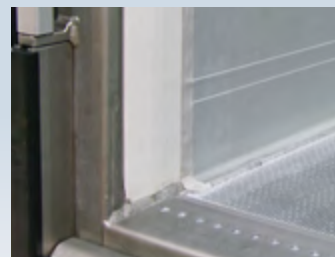
Stable temperature connection. Improved attachment of the portal to the rear of the trailer.
