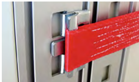
Special lashing straps can also be used in the double-decker rails for additional load securing.
