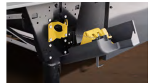
Landing gear with ferry lashings and storage compartment for the securing wedge.
