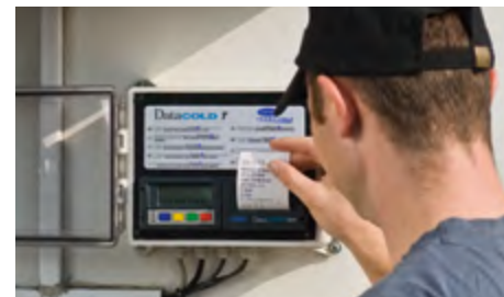
Conventional or digital temperature recorders for indisputable proof in accordance with DIN EN 12830.
