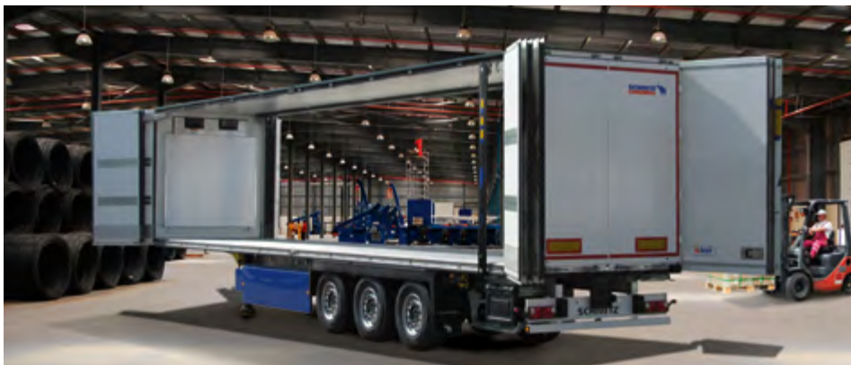
Two-sided folding wall – enables flexible loading from three sides. Can also be combined with a refrigeration unit at the bulkhead as S.KO FW COOL.
