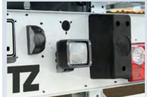
Working spotlight for safe handling at the rear portal.
