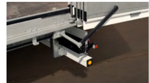
Securing of the folded doors at the rear portal frame.
