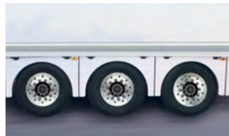
Cladding on the chassis reduces wind resistance, the wheel nuts and wheels remain directly accessible.
