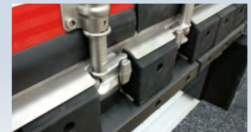
A double rubber buffer rail* at the rear protects the body and the espagnolettes.
