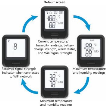
Users can press the button on a WiFi-500 sensor to cycle through different information screens (WiFi-502 screens are shown above).
