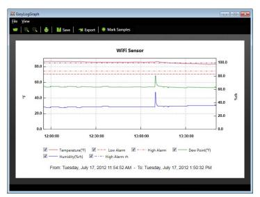
Users can select the WiFi-500 Sensor Series data to display using the EL-WiFi software (WiFi-502 data graph shown above).
