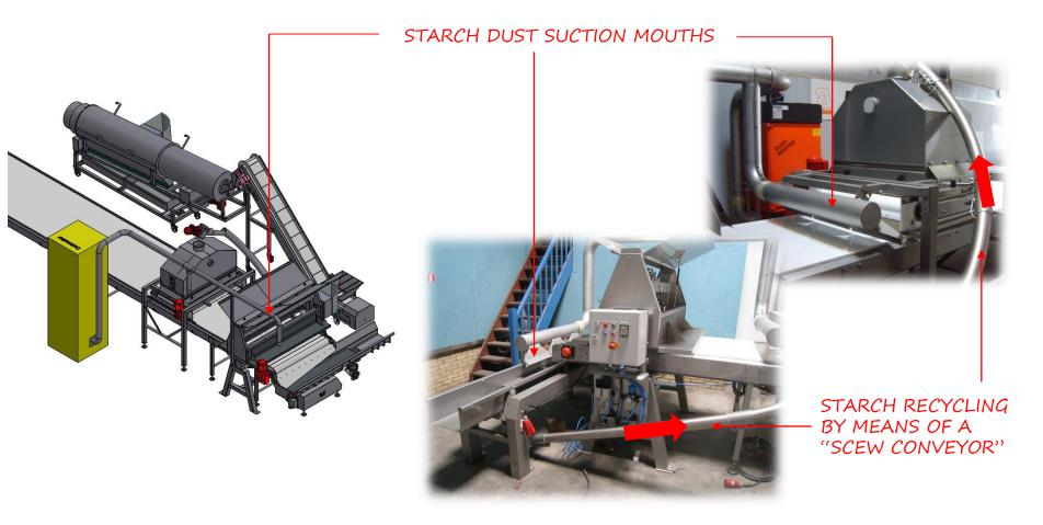
STARCH FROM THE CROSS SHAKER AND DE-STARCH DRUM IS RECYCLED TO THE TOP STARCH DEPOSITOR. THE BOTTOM STARCH DEPOSITOR HAS "NEW FRESH" STARCH
