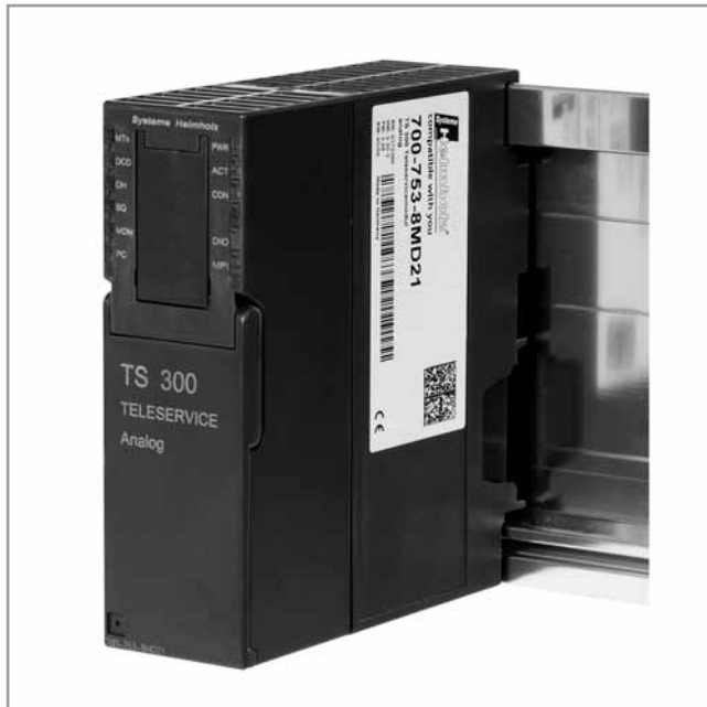
TS 300, Teleservicemodule for the PLC-Rack
