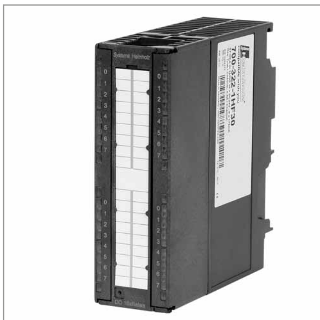
DEA 300, Digital Output; Relays Bistable
