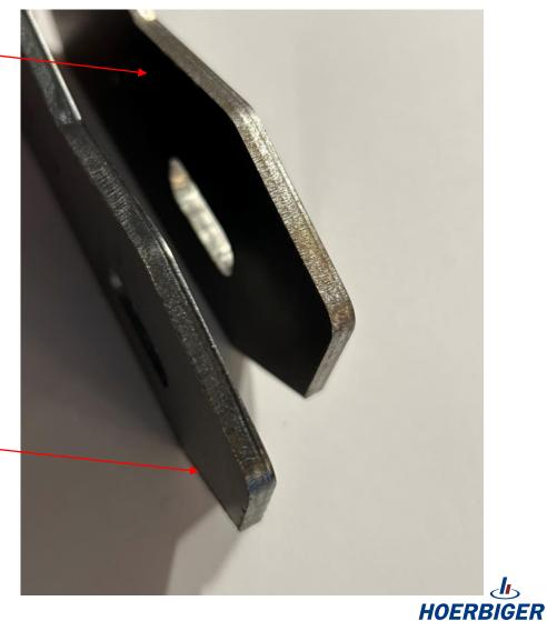
left: mild steel t = 10 mm; p = 7 bar, v = 4800 mm/min (10 kW) MIX GAS
