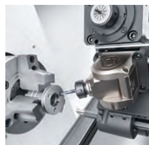
Inclined hole machining with the universal holder
