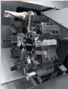
2-axis turning specification 10-station turret
