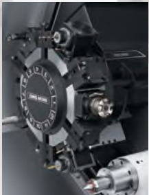
Milling + Y-axis specifications / Milling + Spindle 2 specifications 12-station turret
