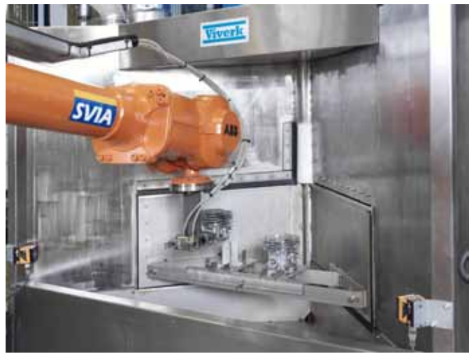
Robot laddar/lossar cylindrar.
