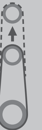
Dimensione nastri abrasivi (sviluppo) 2620mm Abrasive belt (length) 2620mm Dimension de la bande abrasive (développement) 2620mm
