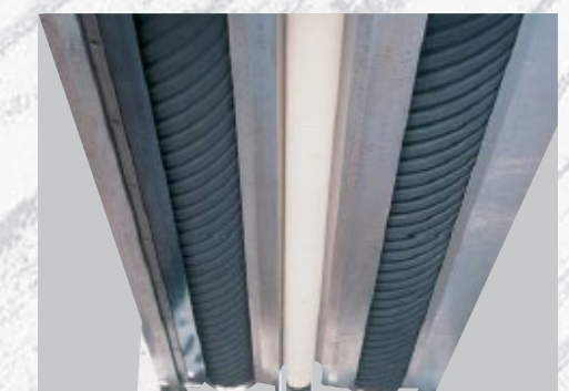
Dimensione nastri abrasivi (sviluppo) 2620mm Abrasive belt (length) 2620mm Dimension de la bande abrasive (développement) 2620mm
