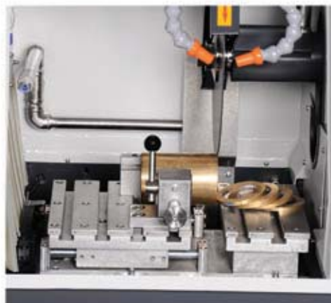
Multi-slice automatic serial cutting of plane parallel sections
