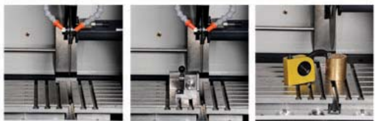
Large cutting chamber with various clamping devices
