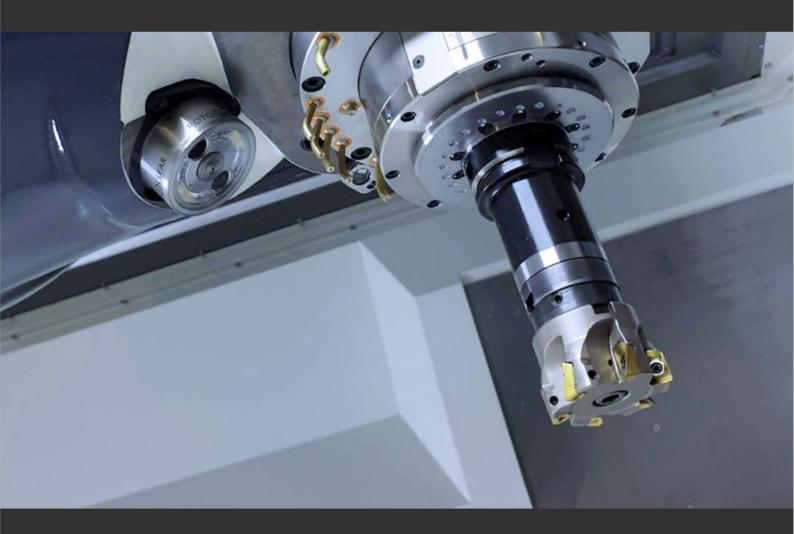
The Rotoclear camera is a camera system that was developed for extremely harsh conditions in machine tools.
