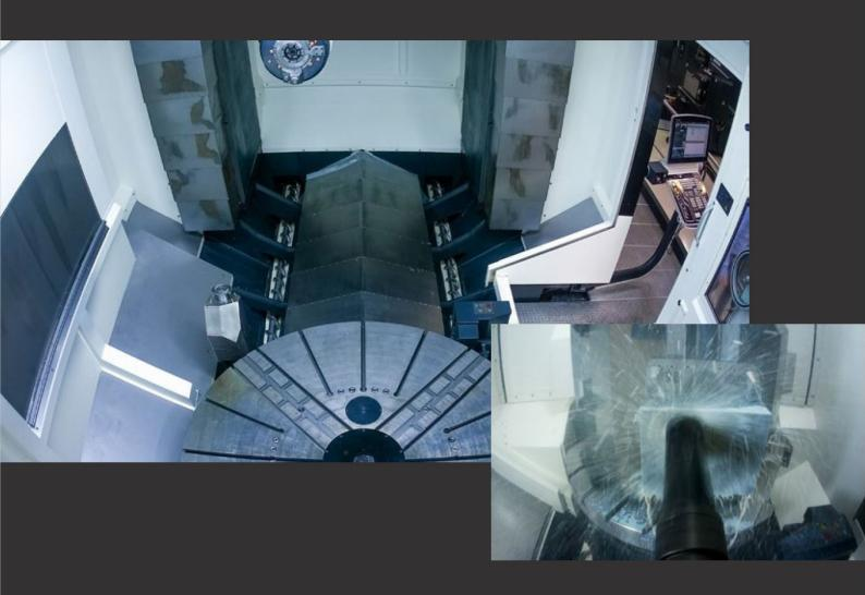
The Rotoclear camera with its rotating window can be mounted in the working space or directly on the spindle head. It is optimally equipped for the movements and accelerations encountered there.
