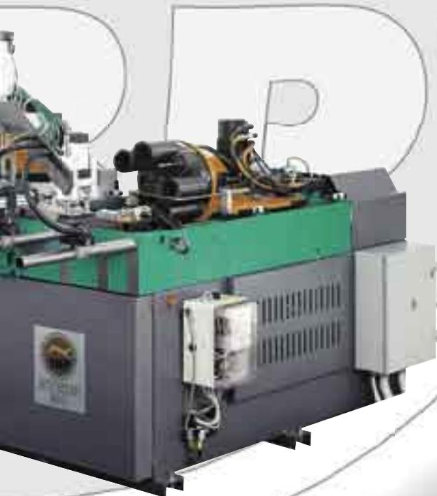
Simplicity of use is the most evident feature of the PEDRAZZOLI IMS multi-axis control. Programming is intuitive and guided by explanatory help pages which describe in a very detailed manner all the available features. Using the latest version of TOUCH SCREEN the operator only needs to indicate the shape of parts he wishes to produce and the tools and type of material he is using; the machine will optimise all other parameters thus reducing to a minimum the actual duration of work cycle.
