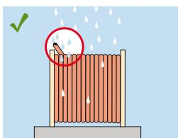
Ensure cable sealing is intact so moisture cannot seep into cable. Report damage.
