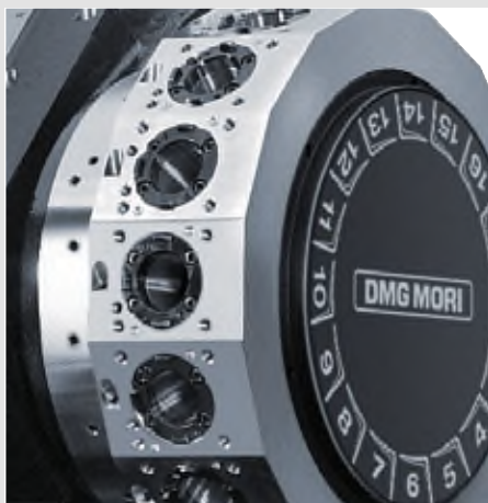
• The photo shows the bolt-tightened turret head
