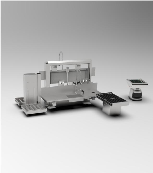
Containers are transported by AGVs (Automated Guided Vehicles) to the roller conveyor in the manual washing area.
