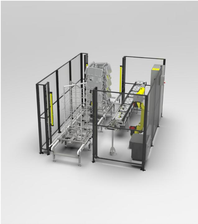
Empty containers and washing racks are automatically transferred into the cell by a conveyor. The washing racks stops on a turntable conveyor that rotates for the robot to fill all four sides of the washing rack.
