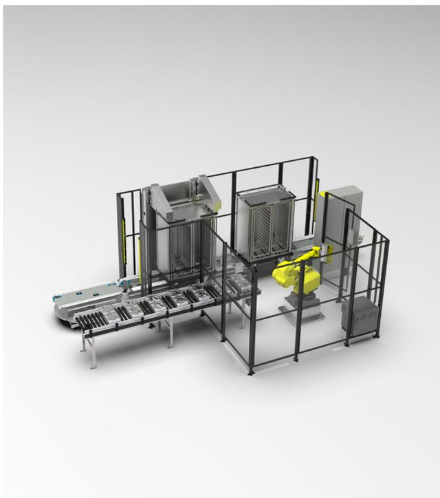
Containers and open transport trolleys are transported into the cell by a conveyor. The containers are picked up by a robot and placed in an open transport trolley.
