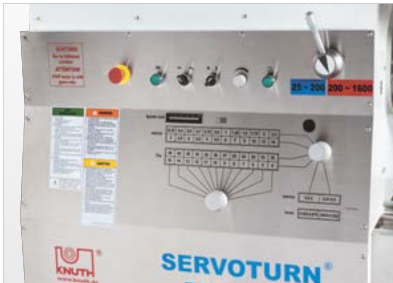
Feeds are selected via 2 rotary switches
