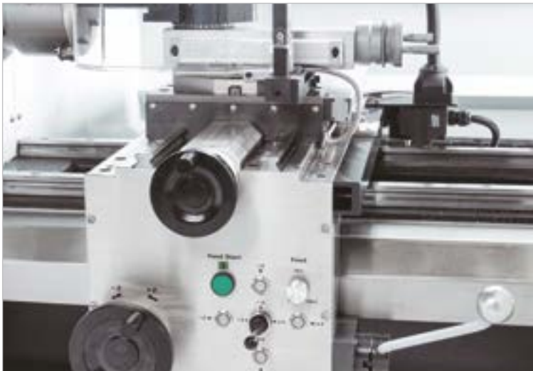
Servo drive technology - including "Teach-in" buttons that allow setting a limit stop at the current position
