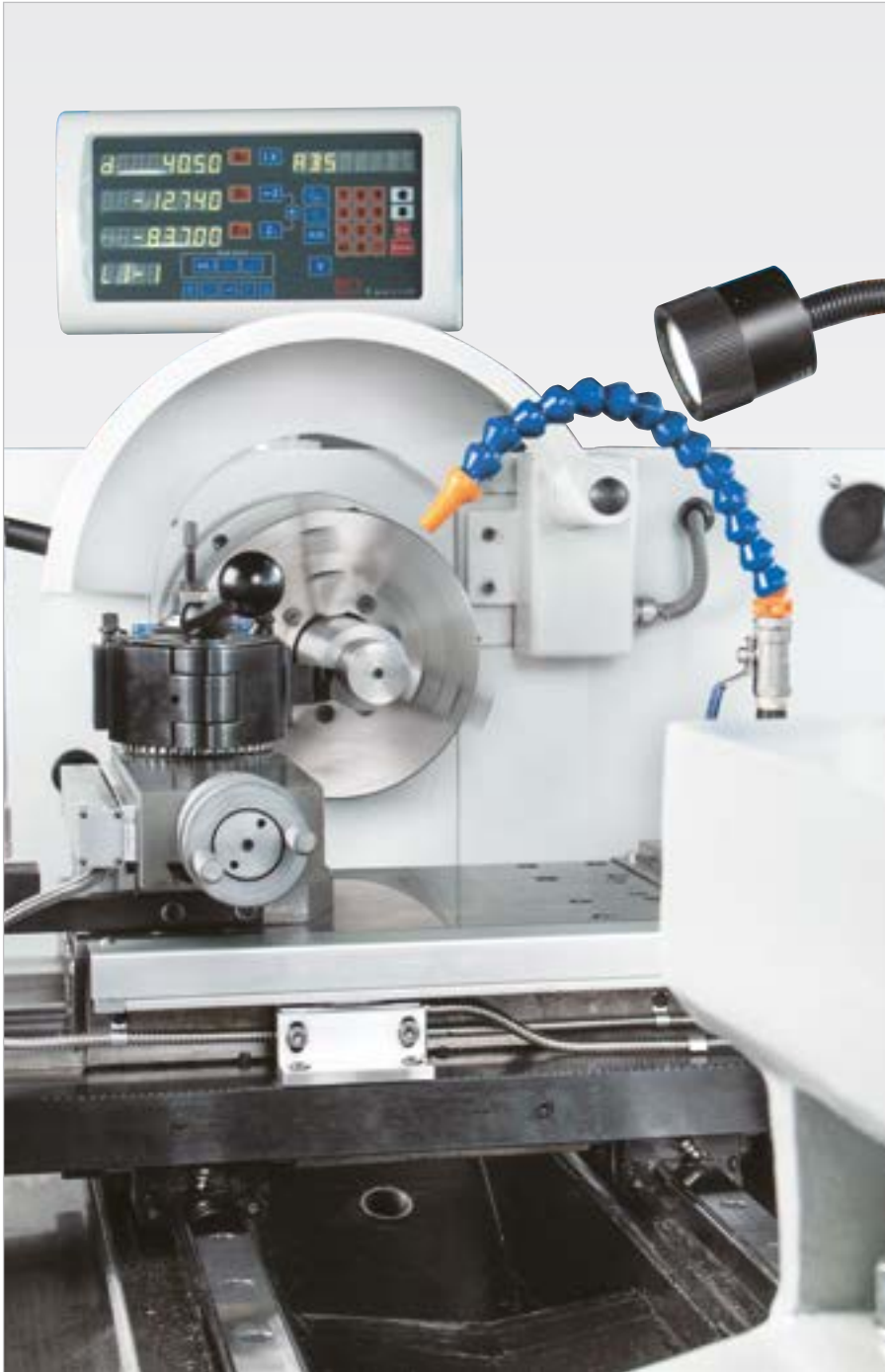
Linear profile rail guides on Z and X
