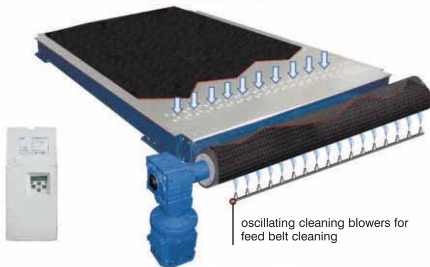
Feed table surface with intakes for vacuum plant
