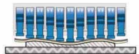
Polishing of deformed and/or uneven pieces
