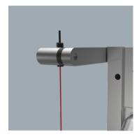
Laser Pointer The Laser Pointer is used to make it easier to select a zero point on the material being worked.
