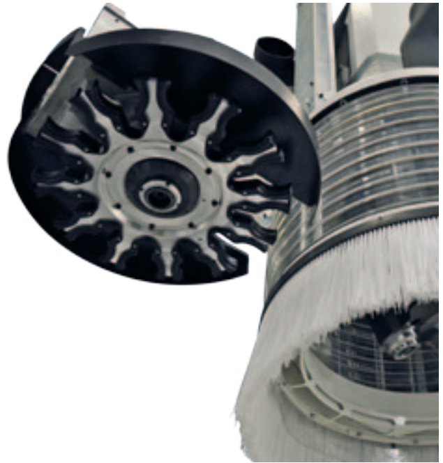
The rapid 12 "on board" magazine fitted directly on the main electro-spindle allows for tool changes in masked time, during the auxiliary drilling or routing.
