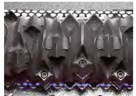
Profile rotor with welded knife carriers in special milled knife pockets (GAZ 62 V)
