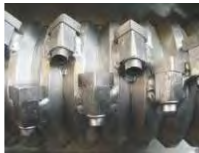
Profile rotor with welded knife carriers (GAZ 62 G)
