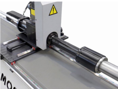
Hydraulic POB clamp NC plane of bend positioner equipped with hydraulic clamp.
