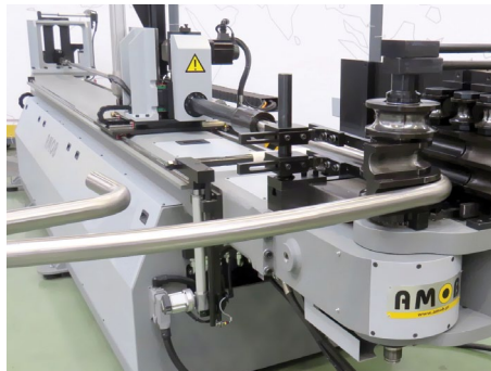
Fixed and variable radius All Ce CNC R models have multi-stack, fix and variable radius capability.
