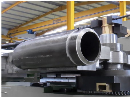
Quick tool changing In order to reduce setup times, all CH-HD features quick tool changing.
