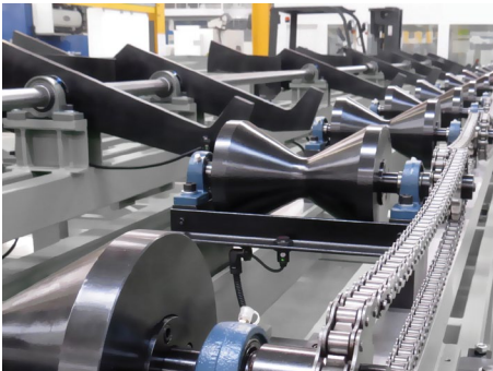
Rear and front tube loading system Integrated loading/unloading systems can also be added.
