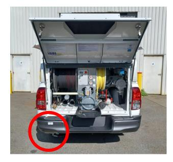
The 12 CV hydraulic system is conceived to drive a transfer pump.
