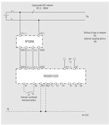
$^{\star}1)$  Auxiliary voltage  $\rm U_{H}$  (A1(+)/A2) ) can also be sourced from the monitored voltage system. The voltage range of the auxiliary supply has to be taken into account.
