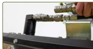
Hydraulisk snabbkoppling (standardutrustning)
