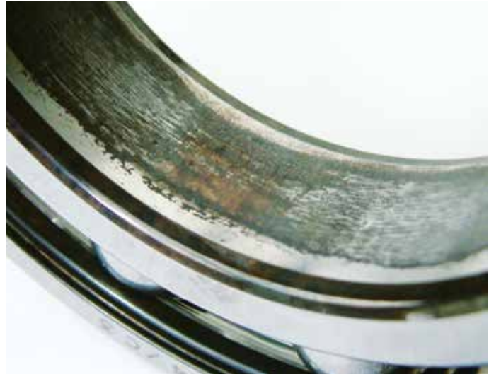
Fretting corrosion on inner ring
