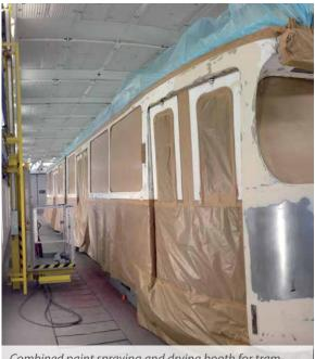
Combined paint spraying and drying booth for tramways and buses
