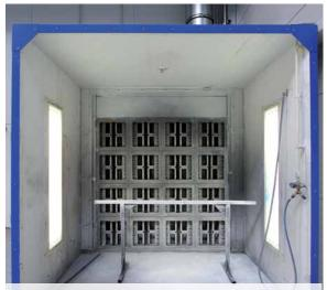
Open face spray booth for the coating of attachment parts of utility vehicles
