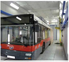
Combined paint spraying and drying booth with lifting platforms
