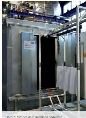
"DARC" furnace with overhead conveyor
