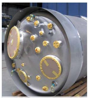
Stainless steel tank blasted with glass beads prior to its coating
