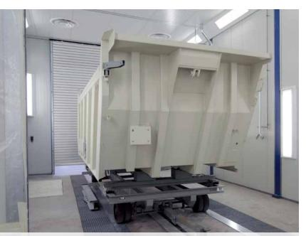
Work piece transport device connected to the floor-mounted chain conveyor in a paint spraying booth
