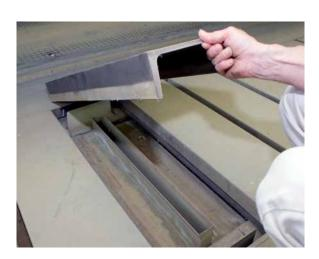
The heavy duty impact separators are the first step of our two stage paint separating system. Due to their special construction, heavy transport devices can drive on the impact separators without problems.
