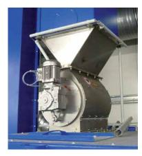
Double magnetic separating roller for the separation of ferrous and non-ferrous blast media or material residues
