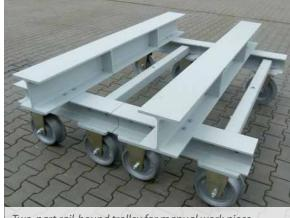
Two-part rail-bound trolley for manual work piece transport
