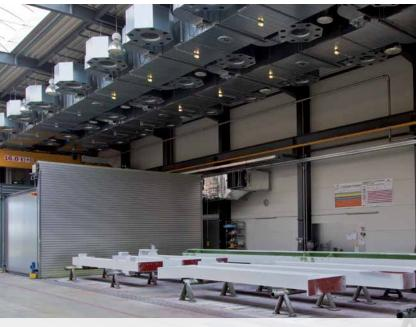
Open-space paint spraying system for steel components and steel structures
