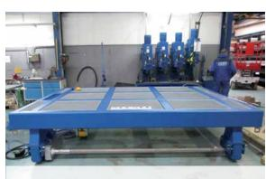
Electrically driven rail-bound trolley with lifting table
