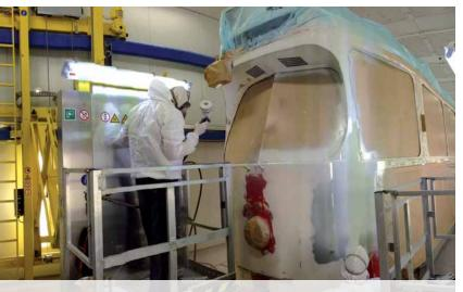
Sidewall scissors-type lifting platforms in a paint spraying booth for trams
