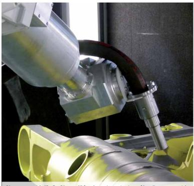
Blastroom with "ReCo-Blaster "" for the paint stripping of landing gears with plastic abrasive
