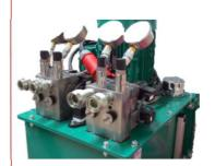
Customized power unit with BIERI pump and applicationspecific valve blocks
