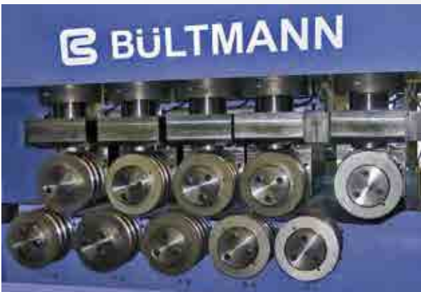
10-Rollen-Vorrichtmaschine für Edelstahlstangen 10-roll pre-straightening machine for special steel bars
