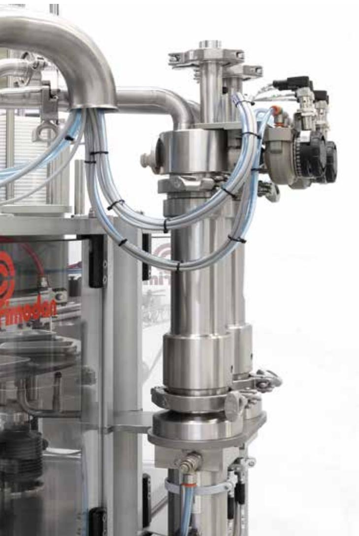
*The PRIMA filling and sealing machines are constructed for filling liquid and semi-liquid products. The machines will fill and seal ready-made cups.*
