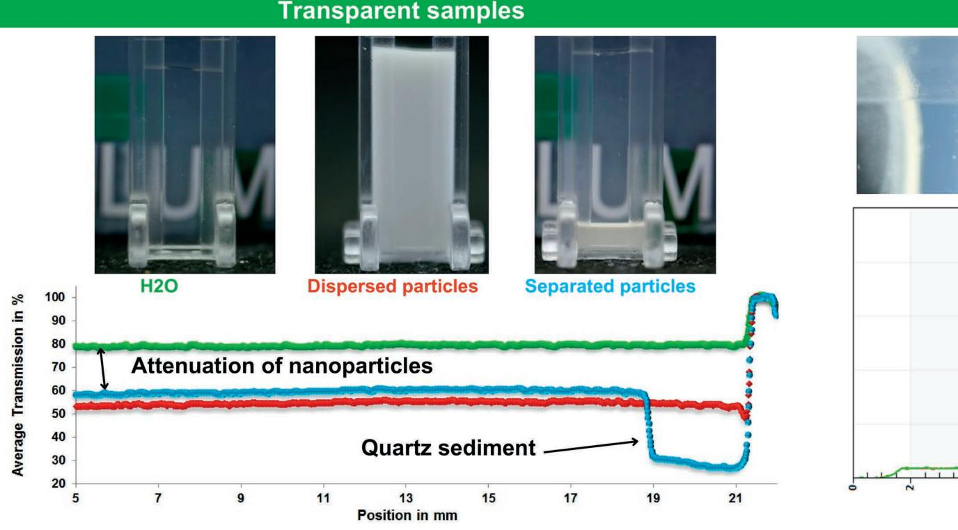
Detection of nanoparticles in supernatant of suspension consisting of 10 % Quartz + 30 % w/w Koestrosol® (15 nm) in water after accelerated separation (10 min at 25°C, RCA = 2300 g)
