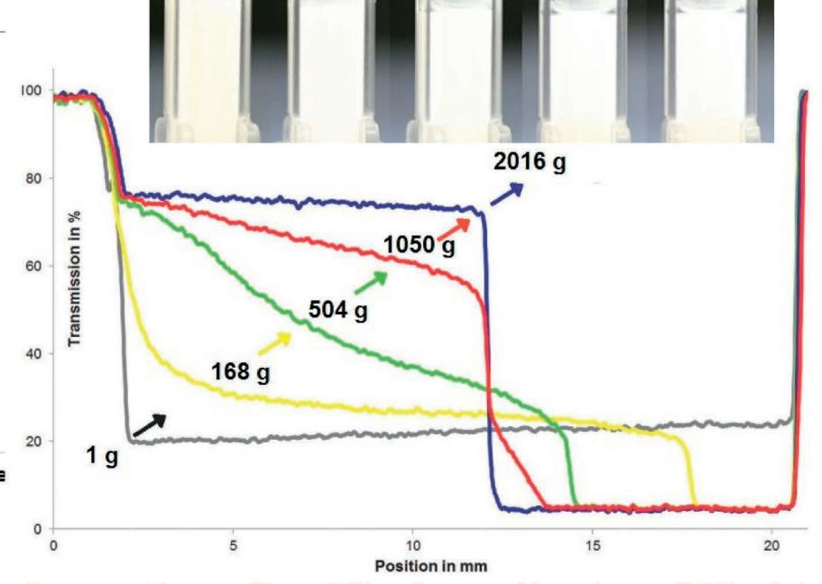
Concentration profiling of filler dispersed in polymer (61% m/m) with LUMiReader X-Ray after accelerated separation for 60 min at 25°C, RCA = 168 g to 2016 g
