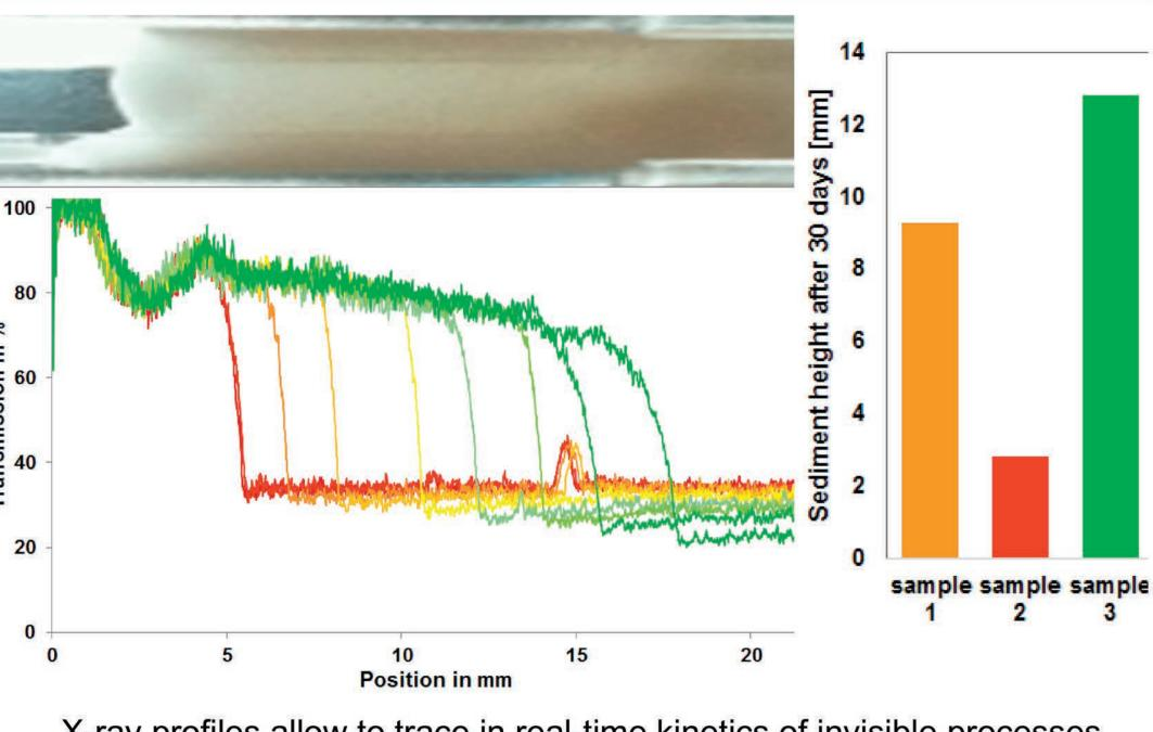
X-ray profiles allow to trace in real-time kinetics of invisible processes. Separation of a filler inside an adhesive matrix (earth gravity). Right comparison of 3 adhesive formulations.
