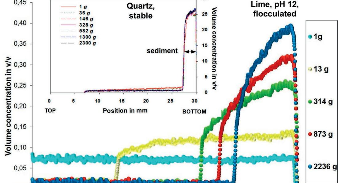
Sediment packing profiling by X-ray after consolidation (different centrifugal forces and particle interaction)
