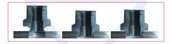
Nut is captivated by pressing on head, which causes the shoulder under the head to reduce the hole diameter in the sheet.
