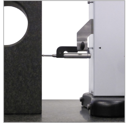
Perpendicularity measurements with electronic probe (TA-IH-126, TA-MS-101)
