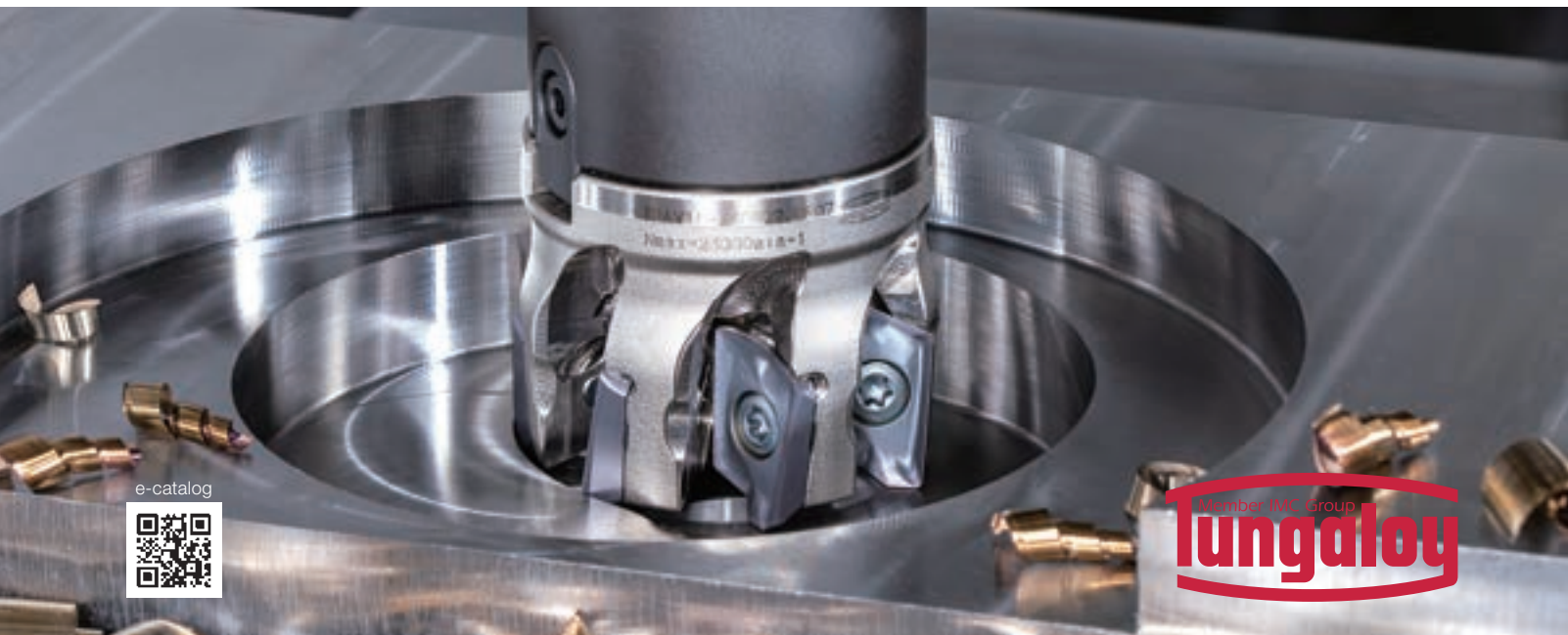
AV*T18 Max. depth of cut: 16.5 mm AV*T12 Max. depth of cut: 11.5 mm
