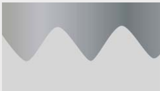
Pre-drilling Ø 17.1 mm
