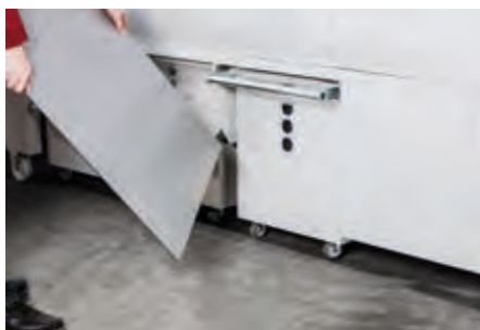
Release the chippings container
