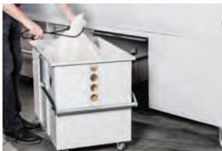
Replace the chippings container
