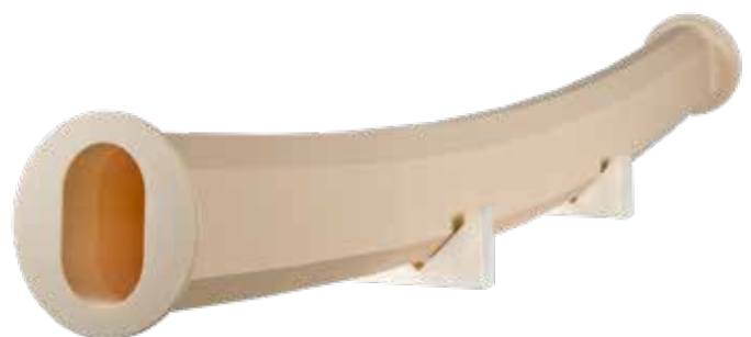
Fig. 2: Curved vacuum chamber with glass-brazed ceramic-to-ceramic joints bending angle: 15°, L 3,200 mm
