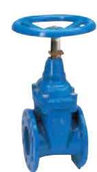
Series 06/35 Flanged gate valve with pin indicator Face-to-face DIN F4 DN 50-400 PN 10/16 Ductile iron
