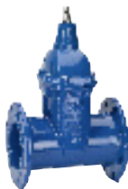
Series 02/60 Flanged gate valve Face-to-face DIN F5 DN 40-500 PN 10/16 Ductile iron
