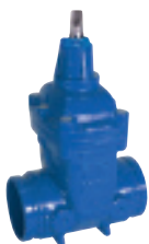
Series 06/38 Gate valve with grooved ends DN 50-300 PN 16 Ductile iron
