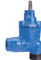
Series 11/00 Service connection angle valve with external thread on inlet and internal thread on outlet DN 25-50 PN 16 Ductile iron
