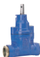
Series 03/65 Service connection valve with tensile screw couplings for PE pipes DN 25-50 PN 16 Ductile iron
