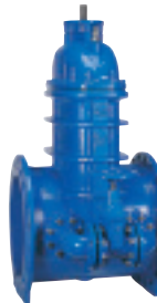
Series 55/30 Flanged gate valve DN 450-500-600-800 Face-to-face DIN F5 PN 10/16 Ductile iron Resilient seated Replaceable stem sealing
