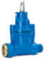
Series 03/85 Service connection valve with tensile screw coupling for PE pipes / external thread DN 25-32 PN 16 Ductile iron
