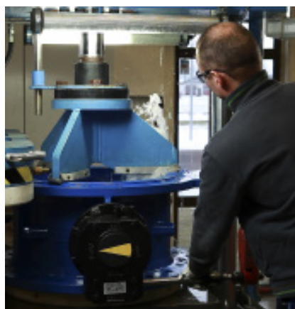
Pressure test of every single valve The hydraulic test is always done from both directions according to EN 1074-1 and 2 / EN 12266.
