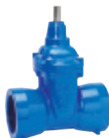
Series 33/00 Gate valve with socket ends for cast iron pipes DN 80-300 PN 16 Ductile iron With internal enamel
