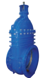
Series 54 Flanged gate valve DN 700-800-900 Face-to-face BS PN 10/16 Ductile iron Metal seated
