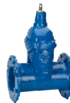
Series 02/75 Flanged gate valve Face-to-face DIN F5 Replaceable stem sealing DN 40-500 PN 10/16 Ductile iron
