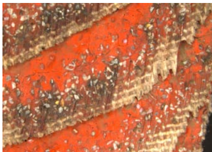
Typical wear pattern with a characteristic shining cooling film (no "glazing").
