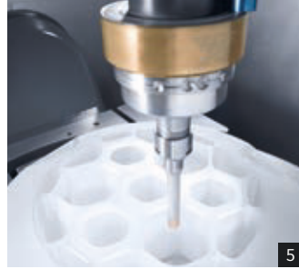
4: Flexible ULTRASONIC technology integration through the HSK-A63 / HSK-A100 interface 5: Thin-walled, lightweight structures in optical components, e.g. made of Zerodur 6: Silicon nitride camera housing for aerial surveillance
