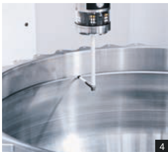
2: Turning with an inclined tool using the A axis* 3: Use of multi-edged tools (up to nine cutting edges)* 4: Measurement cycles for in-process workpiece measurement* 5: Electronic balancing 6: Measurement of turning and milling tools*
