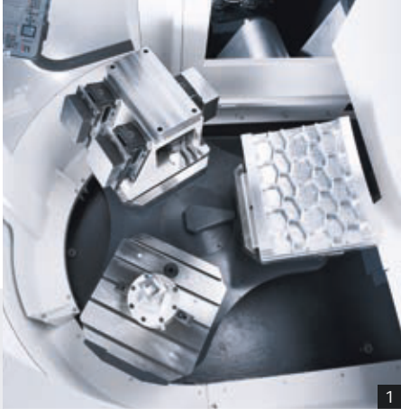
1: Pallet changer for three pallets in a footprint of less than 4 m² with the best accessibility
