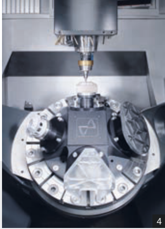
4: Flexible ULTRASONIC technology integration through the HSK-A63 / HSK-A100 interface 5: Thin-walled, lightweight structures in optical components, e.g. made of Zerodur 6: Silicon nitride camera housing for aerial surveillance
