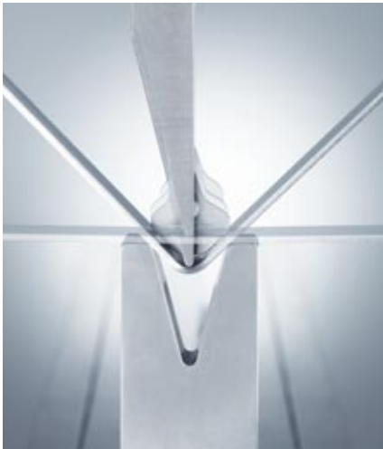
Automatic bending with angle sensor ACB.
