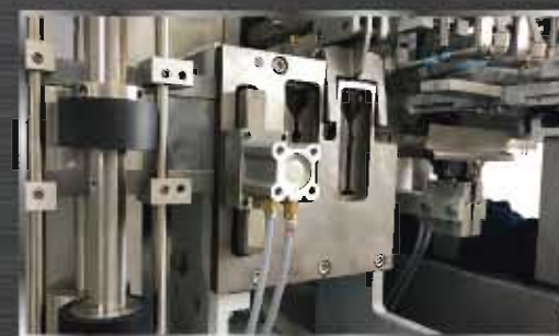
※Shaped punching device.
