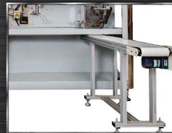
※Front Load Transfer + Outlet Conveyor
