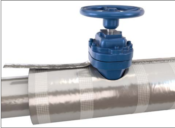
Figure 42: Application of vapour barrier tape
