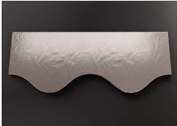
Figure 48: Fabricating the insulation for valve connection
