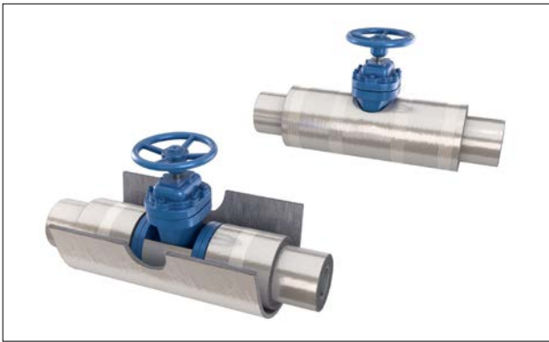
Figure 41: Securing valve body cover with filament tape
