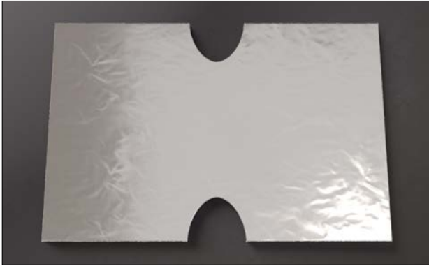
Figure 22: Equal tee fabrication
