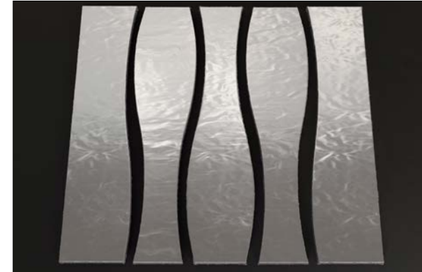
Figure 16: Fabrication of fish-tail patterns
