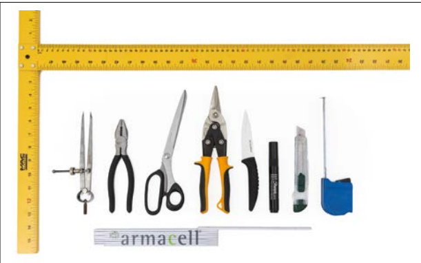
Figure 4: Recommended tools for application of ArmaGel DT
