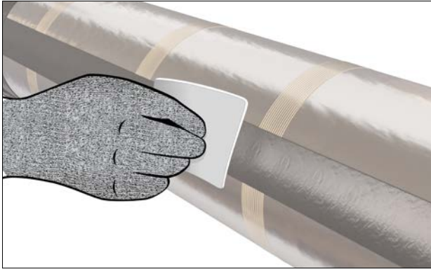
Figure 11: Using a tape card
