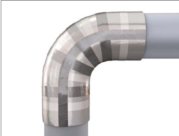
Figure 20: Fully secured vapour barrier tape
