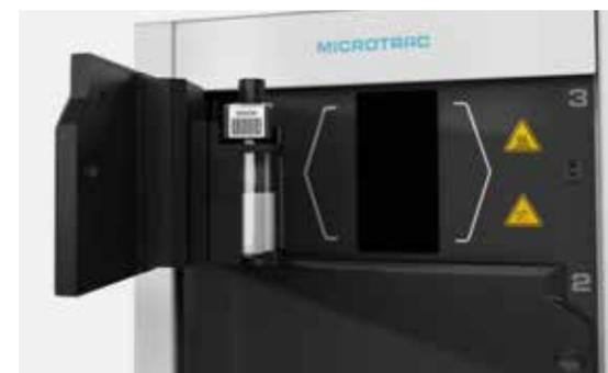
The measurement cell is placed directly in the trap door's sample holder.
