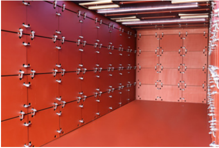
Burst test chamber with sacrificial elements
