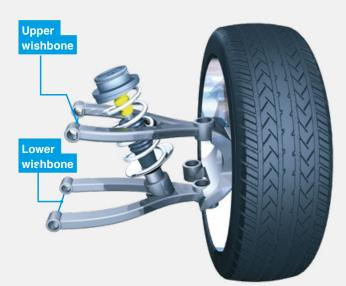
THE STEERING ACTION IS INDEPENDENT OF THE SUSPENSION.
