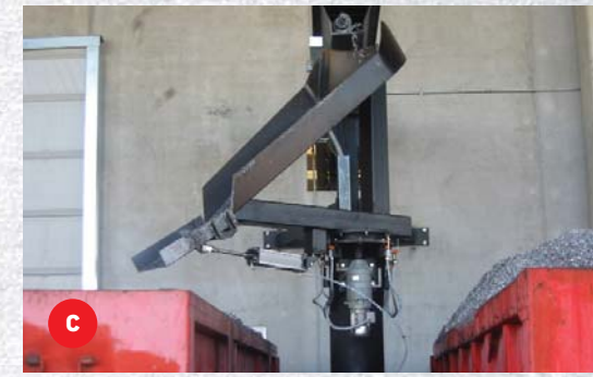
Sistema rotante riempimento contenitori Rotating system to complete filling chip container
