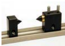
Pair of centers to be mounted on the slide, at adjustable positions
