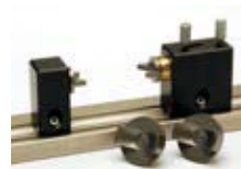
Set of two pairs of hollow cones, to be used with dead centers
