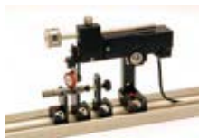
Motor driven device to rotate the part, with friction driving wheel and stepper motor.
