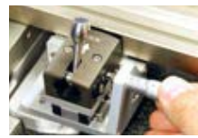
Device for the fine tuning of the slide position, with micrometric head, 0.5 mm/rev pitch, ± 6.5 mm range
