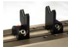
Pair of fixed V blocks (various heights) to be mounted along the slide
